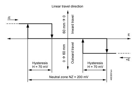
Actuators GBB163.2, (DC 0...35 V) For DC 0...35 V (with characteristic function) the following values apply:
